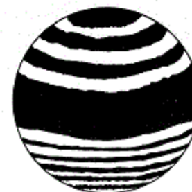
Fig. 109—Oblique residual astigmatism and coma
