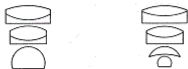
Fig. 105—Microscope objectives (Left) 4-mm dry objective (Right) 2-mm oil-immersion objective
