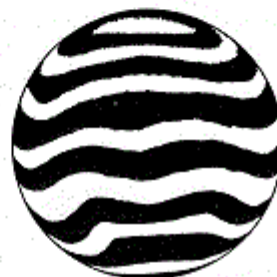
Fig. 108—Axial residual spherical aberration
