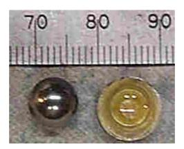
A steel ball was used as a lap although this lap is for a slightly smaller lens than the one pictured . The lens is bonded to an aluminium disk
