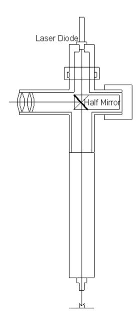
The half silvered mirror is a unit from Surplusshack. It is mounted in a small square tube. I have a quality beam splitter but consider this cheap half silvered mirror perfectly adequate for this use. The cross piece is bored so the mirror unit is a firm push fit. It can then be pushed and twisted into position and a cover screwed in place.
