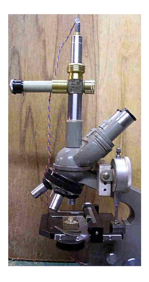
1/ The surface under test can be seen in this photograph. It is a miniature concave piece of F4 glass bonded to a small Aluminium disk for the lens polishing machine. It is visible on the stage. The stage has fine X and Y movements. This makes operation a pleasure.
