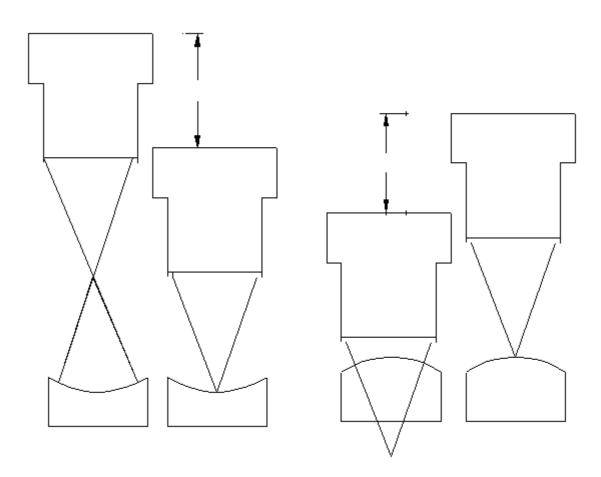
Note that the microscope objective is always further from a concave surface. This means that longer focal length objectives must be used for convex surfaces.
