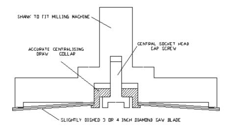
The main advantage of this generating tool is the ease of blade changing. You will be surprised, however, how long a blade lasts and the quantity of glass it will shift. A photograph is included later.
