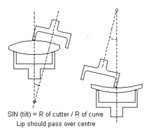
The principle of generation using this method is illustrated above. The setup may be accomplished by
