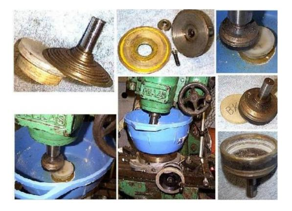
Visible is a disk of Aluminium to which the lens has been waxed. Wax alone is not strong enough. Beeswax and Rosin mined works. The centre of the disk has been relieved to form a cup.
