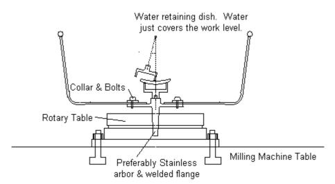
Mill requires tilting head or alternatively a tilting table attachment
