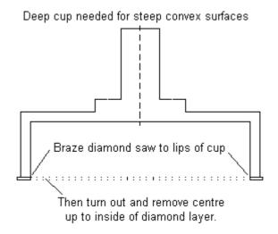
Turning out the centre can be interesting. Apart from unbearable singing of the blade, the diamond chips make mincemeat of a lathe tool if the cut is taken too far. But a HS tool is quick to sharpen so it's no big deal. Singing may be reduced by placing putty or plasticene on the blade.
